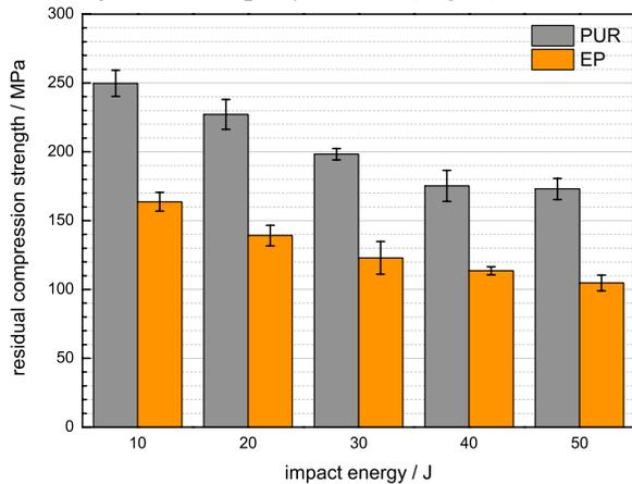
**Figure 2: Residual static compression strengths after different impact loadings**
