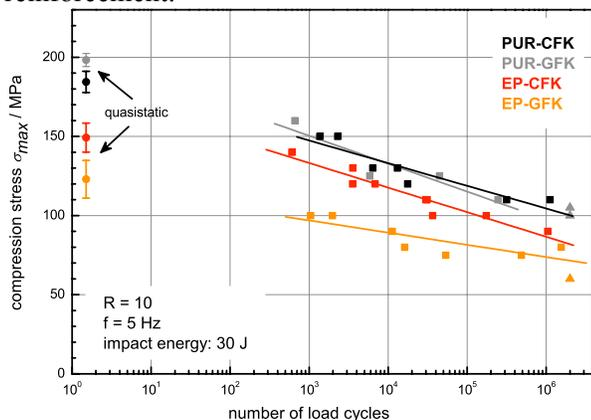
**Figure 3: Compression S/N curves of glass and carbon fibre reinforced polyurethane and epoxy after 30 J impact loading**
