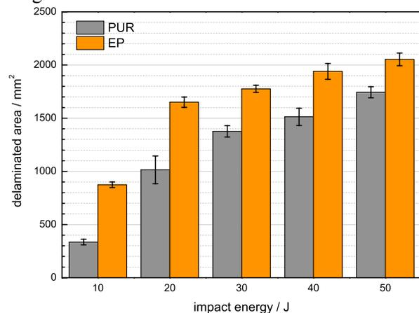
**Figure 1: Delaminated areas of epoxy and polyurethane based glass fibre reinforced laminates after different impact loadings**
