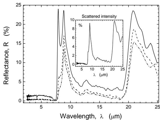
Figure 3: IR reflection from the S1 template at different  $\theta_{inc}$ ; dash-dotted line –  $20^\circ$ , dashed line –  $35^\circ$ , solid line –  $50^\circ$ . Inset – the scattered  $R$  with  $\theta_{inc} = 35^\circ$  and  $\theta_{ref} = 45^\circ$ .
