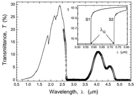
Figure 2: Normal transmission spectrum from the S1; inset – the visible spectrum from the S1 and S2 templates; lines – the Varian Cary 500, squares – the Bruker Vector-22 data.
