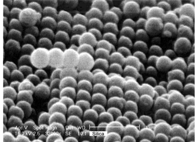
Figure 1: A SEM image ( $\times 3200$ ) of the S1 template.
