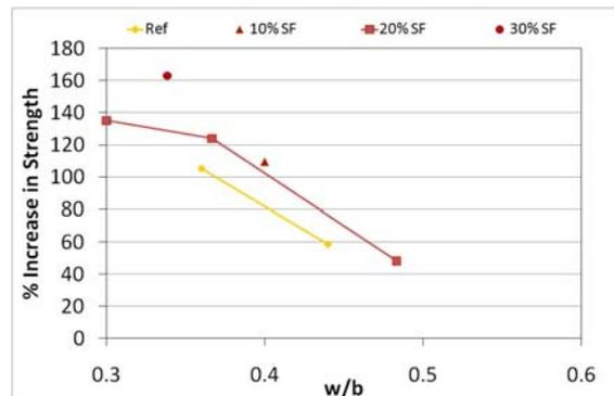
Fig. 4 % increase in compressive strength compared to reference sample with w/c=0.58
