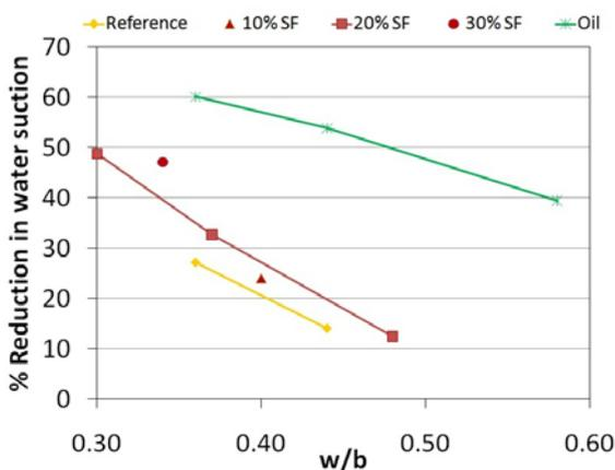
Fig. 2 % reduction in one sided water suction at 4 days compared to reference sample with w/c=0.58
