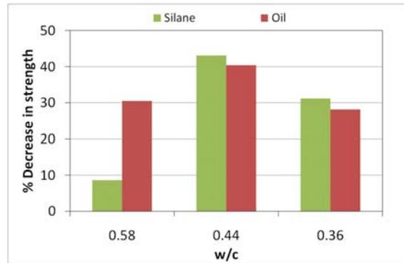
Fig. 3 % reduction in compressive strength compared to reference samples with the same w/c.
