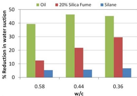
Fig. 1 % reduction in one sided water suction at 4 days compared to reference samples with the same w/c.
