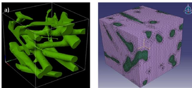
**Fig. 2.** Real microstructure of  $Al_2O_3$ -Cu IPC from micro-CT images (metal phase) (a). FE representation in ABAQUS via Simpleware ScanIP/ScanFE (b).
