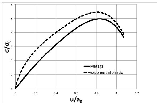
**Fig. 5.** Normalized  $(\sigma - u)$  relationship in metal ligament derived numerically by FEM;  $\sigma$  and  $\sigma_0$  denote the nominal and the yield stress of the ligament material (Cu);  $a_0$  is the ligament's initial radius. Solid line depicts the analytical solution by Mataga [4].
