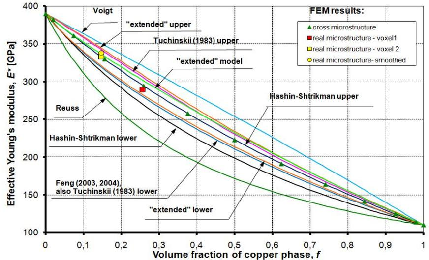
**Fig. 3.** Effective Young's modulus of  $Al_2O_3$ -Cu IPC: Analytical and numerical models and CT measurements results.
