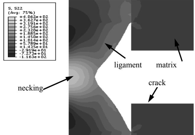
**Fig. 4.** Axial stress distribution in metal ligament at large plastic deformation (necking) and delamination from the matrix; numerical solution by ABAQUS.
