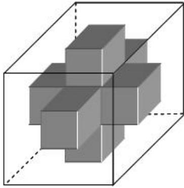
**Fig. 1.** Cross model of interpenetrating microstructure of IPC.
