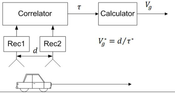
Fig. 1 Principle action of the speed sensor [1]
