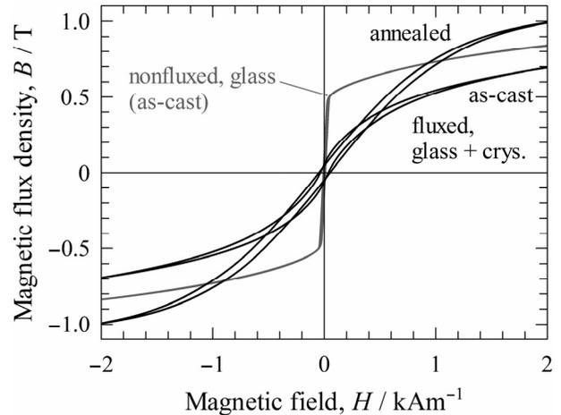
Fig. 2 Hysteresis curves of ring-shaped bulk specimens.
