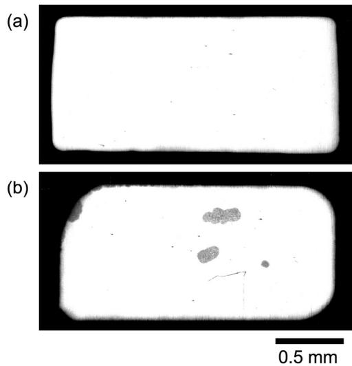
Fig. 1 Optical micrographs of cross sections of etched (a) fluxed and (b) nonfluxed specimens in an as-cast state.
