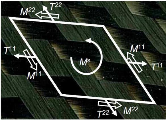
Fig 1. . Unit woven cell submitted to tension, in plane shear and bending
