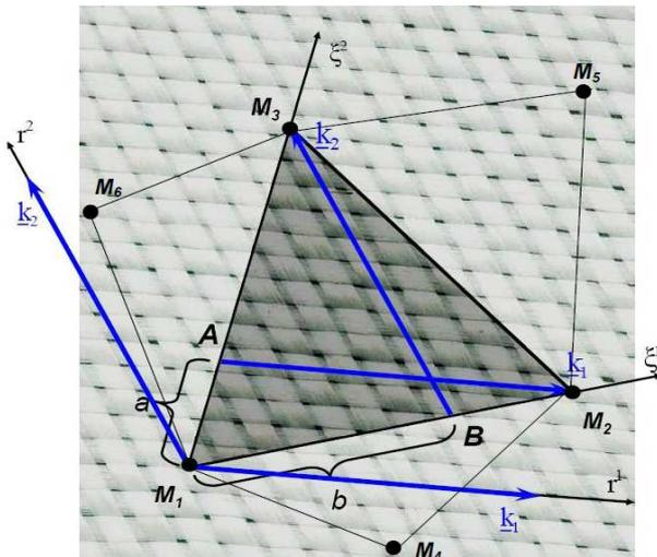
Fig 2. Three node finite element made of woven cells
