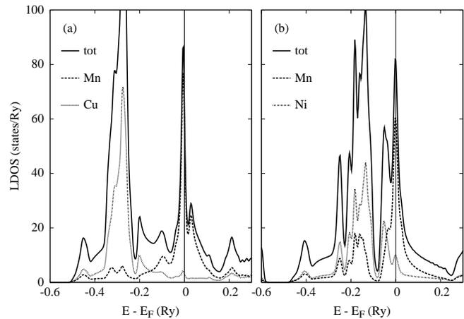
**Figure 1:** Total and component resolved densities of states, per formula unit and spin, for nonmagnetic Heusler alloys: (a) ordered  $\text{Cu}_2\text{MnSn}$ , (b) ordered  $\text{Ni}_2\text{MnSn}$ .
