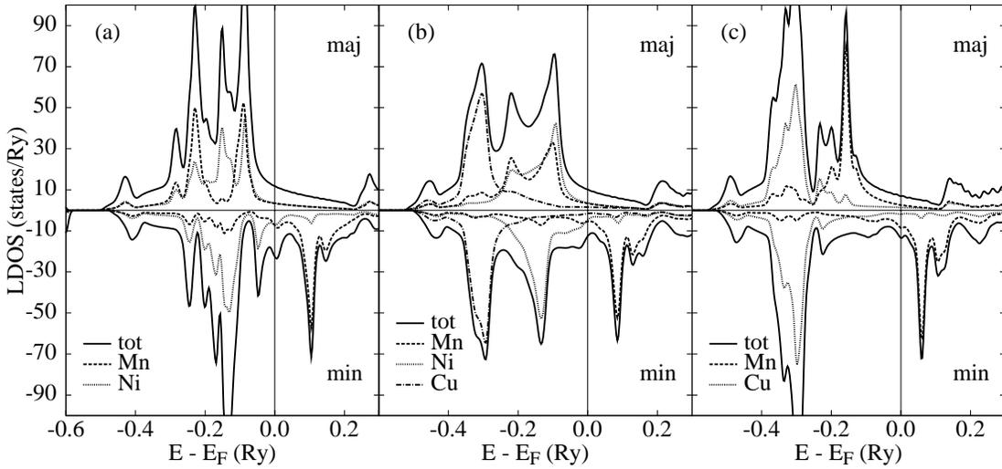
**Figure 2:** Total and component resolved densities of states, per formula unit and spin, for ferromagnetic Heusler alloys: (a) ordered  $Ni_2MnSn$ , (b) disordered  $(Ni_{50},Cu_{50})_2MnSn$ , and (c) ordered  $Cu_2MnSn$ .
