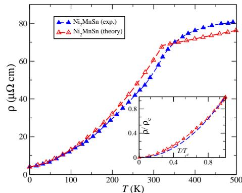
**Figure 7:** (Color online) Calculated and experimental T-dependent resistivities of  $\text{Ni}_2\text{MnSn}$ . Validity of a simple model for the effect of spin-disorder on resistivity (see text) is illustrated in the inset.
