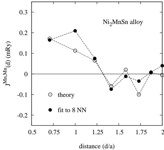
**Figure 5:** Comparison of calculated exchange integrals (present paper, theory) with those obtained from the fit to neutron spin-wave scattering experiment (Table I of Ref. [15], 8 NN fit).
