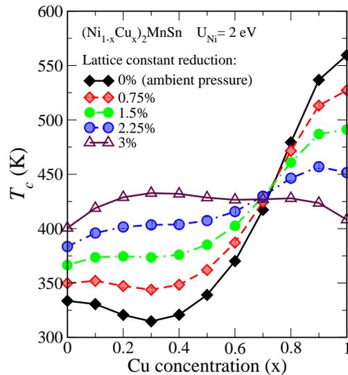
**Figure 9:** The concentration dependence of Curie temperatures (RPA) for  $(\text{Ni}_{1-x}\text{Cu}_x)_2\text{MnSn}$  alloys for ambient pressure and for set of pressures corresponding to indicated reductions of the alloy lattice constant. Model assumes electron correlations on Ni-sites treated in the framework of the LSDA+U method.
