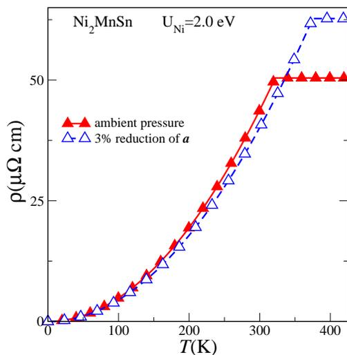
**Figure 10:** The temperature dependence of the resistivity of  $\text{Ni}_2\text{MnSn}$  calculated for the ambient pressure and the pressure corresponding to 3% reduction of the lattice parameter.
