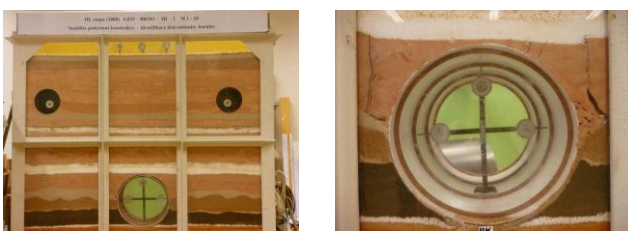
Fig. 3 The model Geo-2008 III Scale 1 : 10: Situation after finishing building of the model (left), Formation of cracks after finishing the tunnel excavation – detail (right)
