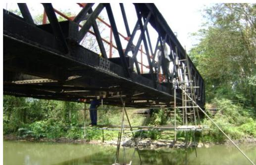
Fig.2 Fixing of displacement gauges to the bridge
