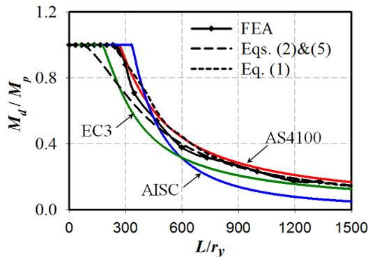
Fig. 1 Comparison of FEA results with the proposed DB solutions and the LTB solutions of the codes
