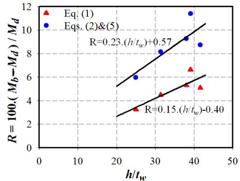
Fig. 2 Reductions in the buckling moments for various web slenderness values
