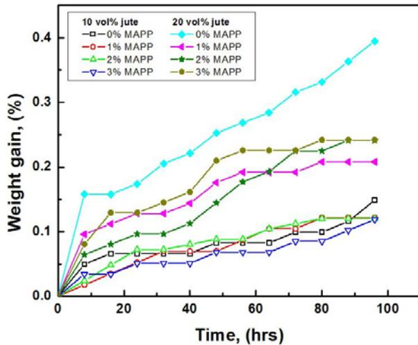
Fig. 1. water absorptions of jute/pp composites
