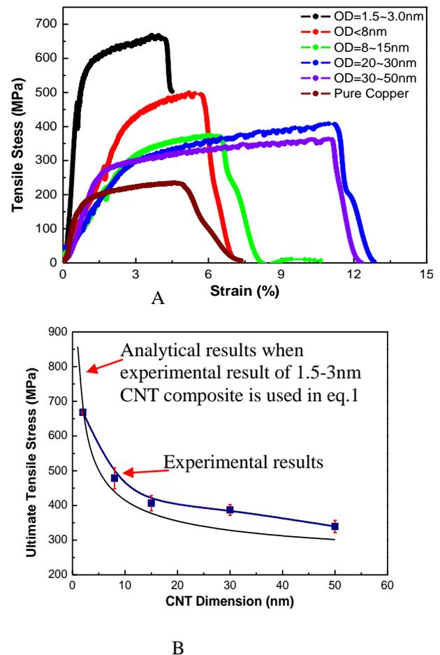
**Fig. 2** Tensile stress-strain curve of pure Cu and Cu/CNT composites with different diameters (A) and averaged tensile strengths versus CNT diameters of Cu/CNT composites (B)
