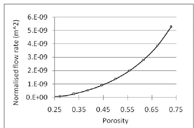
Fig. 1 Mass flow rate at various porosity
