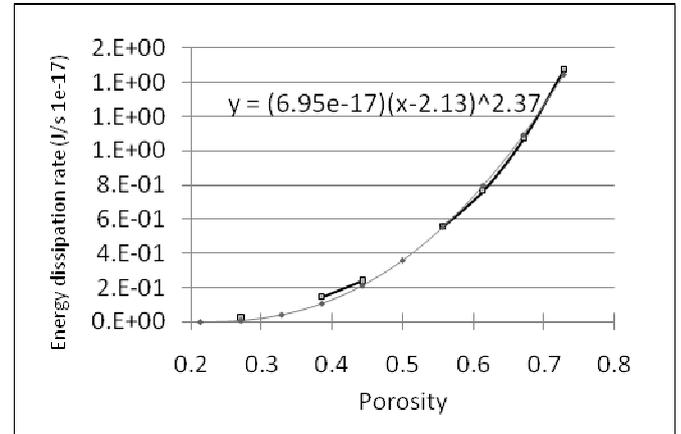
Fig. 3 Homogenized energy dissipation rate by curve fitting
