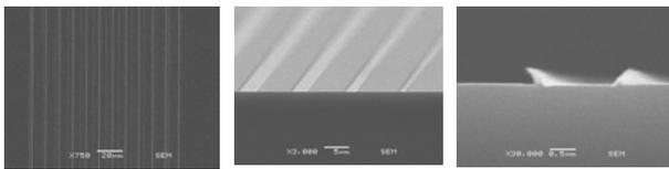
Figure 2. The scanning electron microscope (SEM) photographs of the gold sidewalls pattern.
