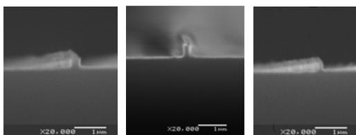
Figure 3. SEM views of the nano-molds with gold sidewalls in different widths.
