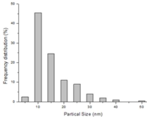
Fig. 2 The particle size distribution of ferrites formed on the silica surface.
