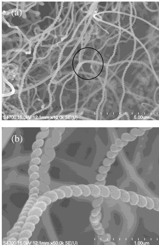
Fig. 3(a) The SEM micrograph of CNCs synthesized by catalytic thermal CVD. (b) The enlarged SEM micrograph as circled on (a).
