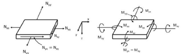
Fig. 2 In-plane, bending and twisting load applied on a laminate
