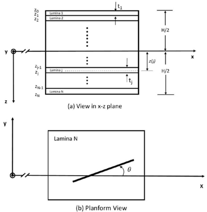
Fig. 1 Laminate nomenclature and definition of surface
