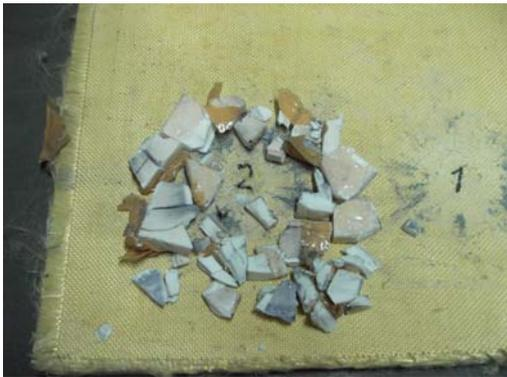
Fig. 3 Kevlar-29 and ceramic plates after an experiment.
