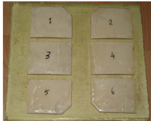
Fig. 1 Kevlar-29 composite laminate and ceramic plates used in experiment.
