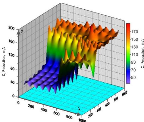
Fig. 3 The reduction of  $C_p$  due to the cyclic load application ( $P = 270$  kN)
