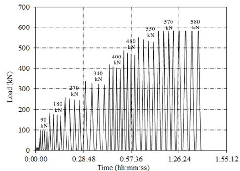
Fig. 2 Loading profile for cyclic loading test
