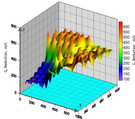
Fig. 4 The reduction of  $C_p$  due to the cyclic load application ( $P = 4800$  kN)
