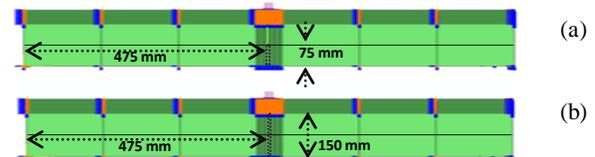
Fig. 5 The influence of the crack height on the spectral response
