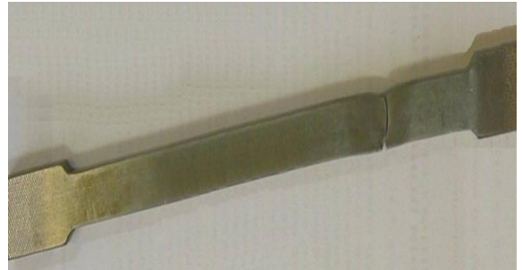
Fig. 1. A photo of the fractured sample of welded joint of 15XCHД steel.
