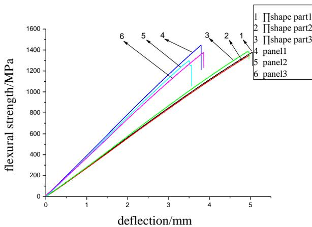
Fig. 2 Stress-strain curves of the samples
