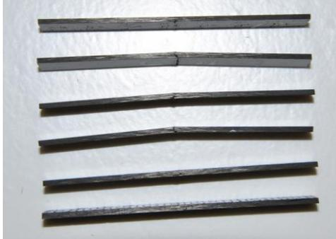
Fig. 3 Bending failure samples
