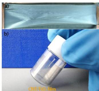
Fig. 2. (a) A free-standing CNT/TiO<sub>2</sub> film on a scaffold. (b) The CNT/TiO<sub>2</sub> film wrapped on a vial.
