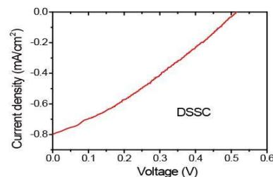
Fig. 4. *I-V* plots of the DSSC based on the CNT/TiO<sub>2</sub> electrode.
