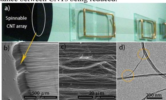
Fig. 1. (a) Carbon nanotube sheet being drawn from a 2-inch spinnable carbon nanotube array. (b), SEM image showing the drawing process of the CNT sheet. (c) SEM image of the CNT sheet. (d) TEM image of the CNT sheet demonstrating that the CNTs are interconnected.
