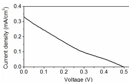
Fig. 3. *I-V* plots of the water-splitting cell based on the CNT/TiO<sub>2</sub> electrode.
