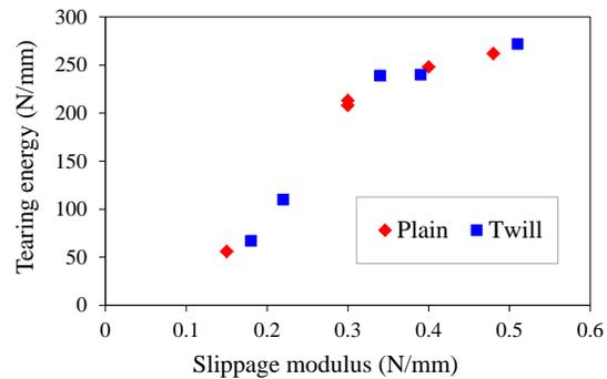
Fig. 3. Variation of the tearing energy as a function of the filling yarn slippage modulus.
