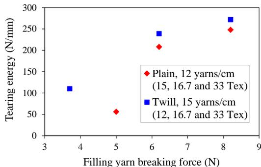
Fig. 2. Variation of the tearing energy as a function of the filling yarn breaking force.
