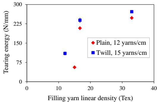
Fig. 1. Variation of the tearing energy as a function of the filling yarn linear density.
