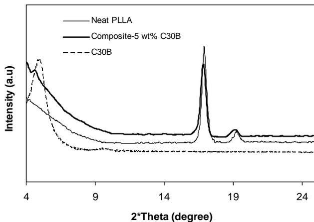
Fig. 1 WAXS pattern of as-received MONT, neat PLLA and PLLA-MONT composite with 5 wt% of MONT
