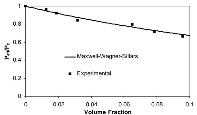
Fig. 2 Comparison of experimental water permeation rate and prediction from MWS model
