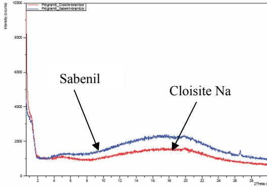
Fig. 2 X-ray diffraction pattern of clay/pristine potato starch composites
