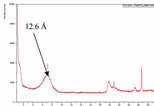
Fig. 1 X-Ray Diffraction Pattern of Sabenil bentonite
