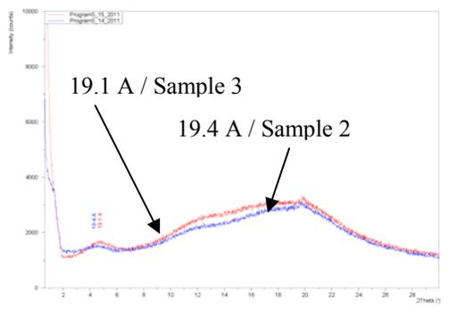
Fig. 3 X-ray diffraction pattern of Cloisite Na/acetylated starches composites
