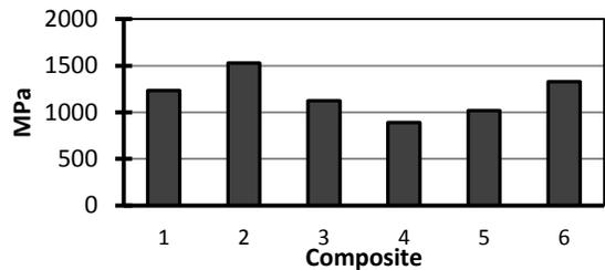
Figure 4 Compression stiffness of the different composite samples.
