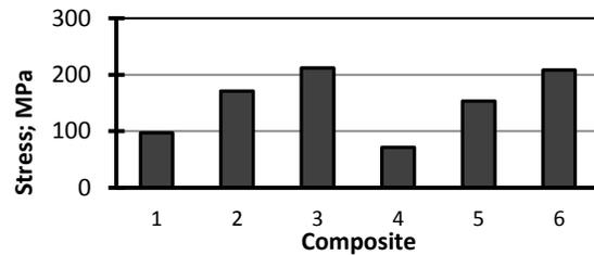
Figure 3 Compressive strength of the different composite samples
