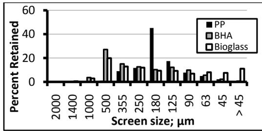
Figure 1 Sieve analysis for the three components.
