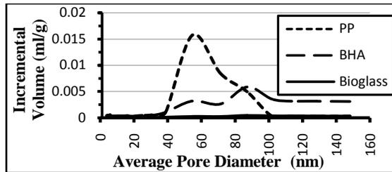
Figure 2 Incremental pore volume versus average pore diameter for the three samples.
