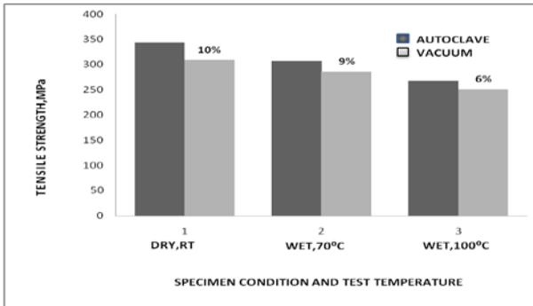
Fig. 1 Effect of Curing Process on Tensile Strength
