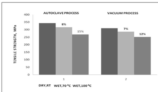
Fig. 2 Effect of Moisture and Temperature on Tensile Strength
