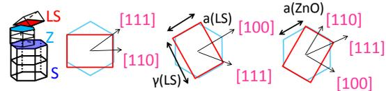
Fig. 5 Possible in-plane orientations of LSMO over-layer on ZnO.  $a(\text{LSMO})//a(\text{ZnO})$ .
