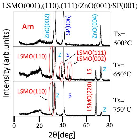
Fig. 2 XRD patterns for LSMO/ZnO/Sapphire. LSMO were deposited at various  $T_s$  shown and  $P_o=1$  mTorr by PL.
