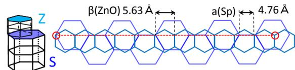
Fig. 4 Possible in-plane orientation of ZnO under-layer on Sapphire.  $\beta(\text{ZnO})//a(\text{Sapphire})$ .
