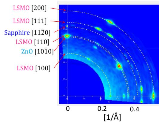
Fig. 3 In-plane RSM for LSMO(110)/ZnO(001)/Sapphire(001). Possible crystalline planes are indicated for spots.
