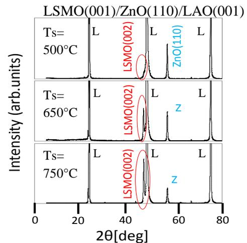
Fig. 1 XRD patterns for LSMO/ZnO/LAO. LSMO were deposited at various  $T_s$  shown and  $P_o=1$  mTorr by PL.
