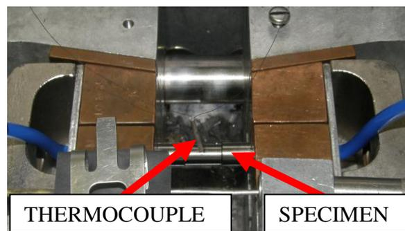
Fig. 1 Test cell with specimen.
