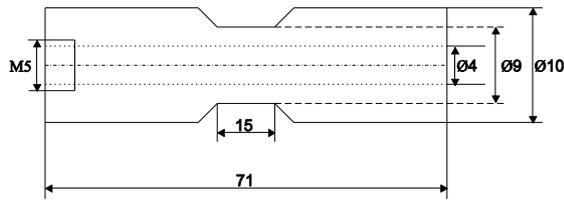
Fig. 2 Dimensions of the specimen (mm).
