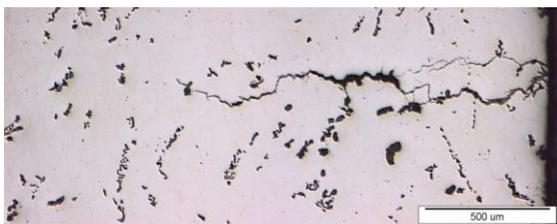
Fig. 4 Image of crack after 1000 cycles at heating temperature 700°C, longitudinal direction.
