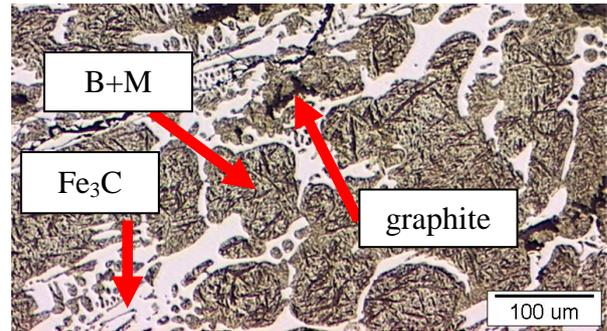
Fig. 3 Microstructure of specimen tested at 700°C for 500 cycles, perpendicular direction.
