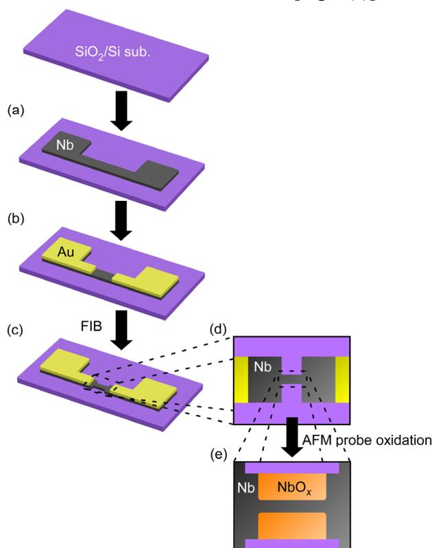
Fig. 1. Device fabrication process.
