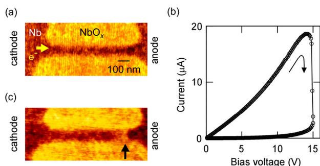
**Fig. 2.** Nb nanochannel device. (a) AFM image taken in the pristine state. (b) Resistive switching. (c) AFM image taken in the HRS after RS. A barrier structure can be recognized in the nanochannel region.
