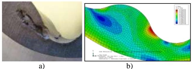
Figure 7. a) Stator lobe hysteretic failure photograph<sup>2</sup>; and b) simulation of lobe stress concentration prediction at the same location.
