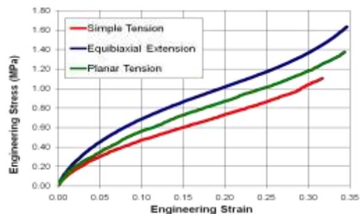
Figure 2. Comparison of mechanical stress-strain behavior of NBR/30vol. % carbon black in uniaxial, equal biaxial and planar extension tests at 66°C.
