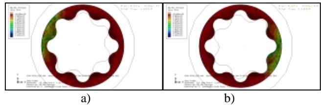
Figure 6. Rotor position and elastomer minimum principal strain in: a) the first; and b) third stator quadrants.
