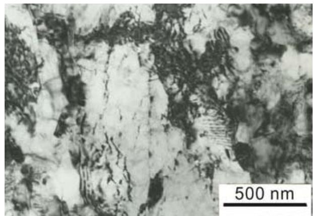
Fig. 5 Substructure CP titanium of the sample after 10 ECAP passes
