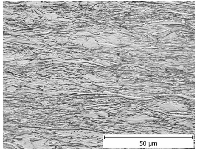
Fig. 2 Microstructure of commercially pure titanium Grade 2 after cold forming (deformation  $\epsilon = 90 \%$ )
