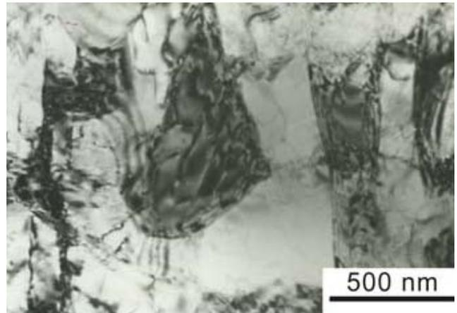
Fig. 4 Substructure CP titanium of the sample after 4 ECAP passes
