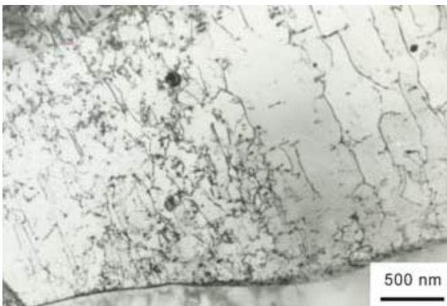
Fig. 3 Substructure of CP titanium Grade 2 in the initial state
