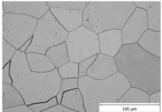
Fig. 1 Initial microstructure of commercially pure titanium Grade 2
