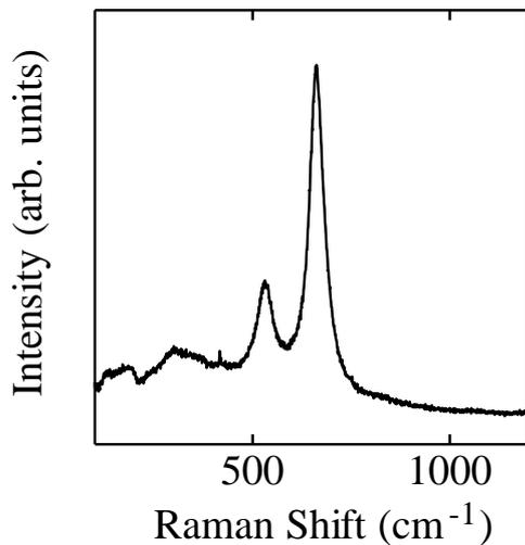
**Figure 2** Raman spectrum obtained at room temperature for the magnetite film on sapphire substrate grown at a substrate of 600°C.
