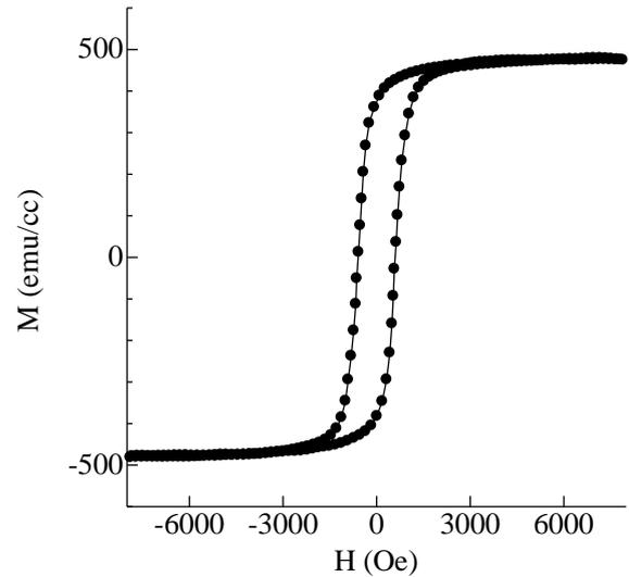
**Figure 3** Magnetic hysteresis loop of the magnetite film on sapphire substrate grown at a substrate of 600°C.
