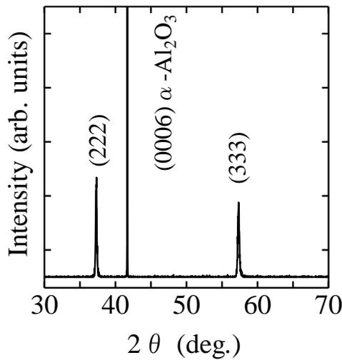
**Figure 1** X-ray diffraction pattern of the magnetite film on sapphire substrate grown at a substrate of 600°C.
