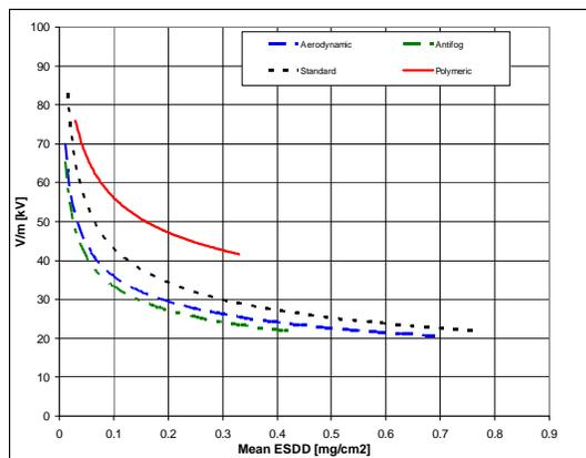
Figure 2. Relative pollution performance of polymeric and ceramic insulators
