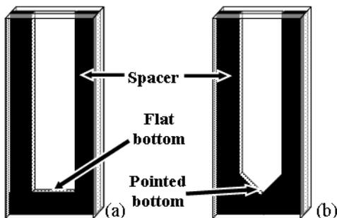
Fig. 1. Schematic illustration of a flat container (a) and an inverted-triangle shaped container (b). Containers have black spacers.
