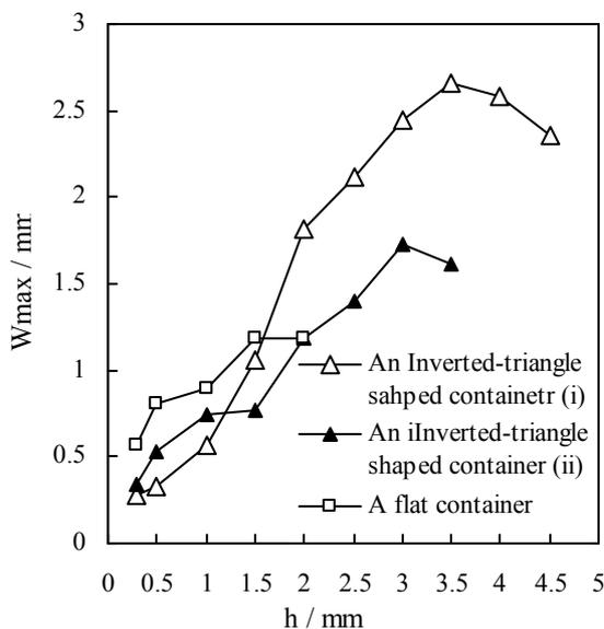
Fig. 2. The widths of the largest grains in the inverted-triangle shaped containers and the flat container.  $h$  is height of the crystals.
