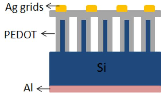
Figure 1: Device structure of the SiNWs/PEDOT heterojunction hybrid cell.
