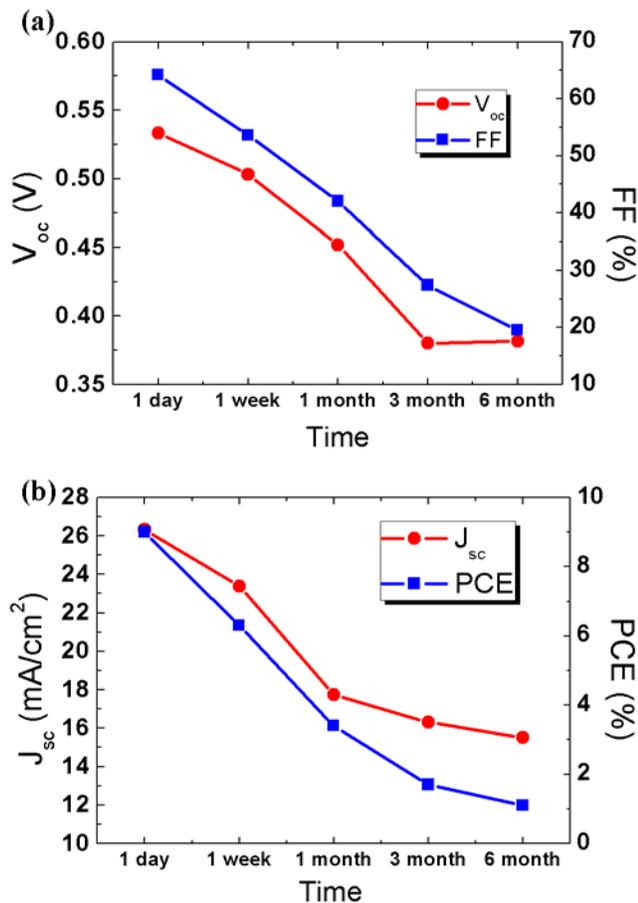
Figure 3: Stability of (a)  $V_{oc}$  and FF, and (b)  $J_{sc}$  and PCE of the SiNWs/PEDOT hybrid cell exposed in the air over time.
