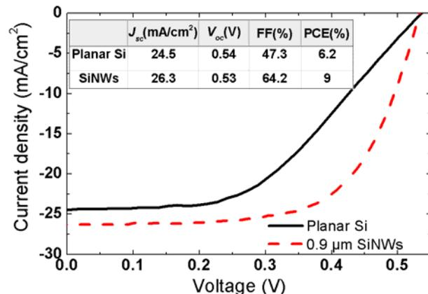
Figure 2: Comparison of current density-voltage ( $J$ - $V$ ) characteristics between a planar Si cell and SiNWs cell under simulated AM 1.5G at 100  $\text{mW}/\text{cm}^2$  illumination.
