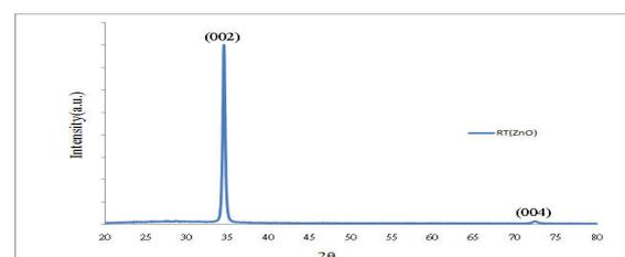
Fig.4: XRD spectra of ZnO film
