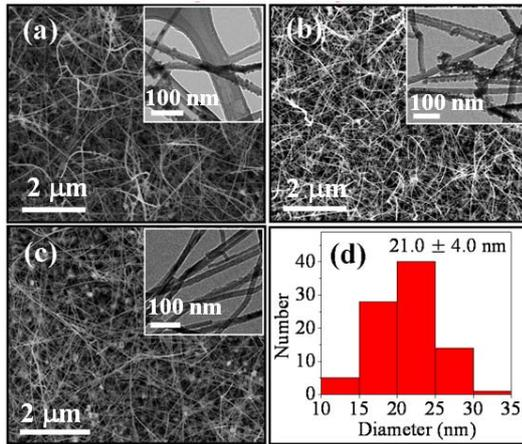
**Figure 2.** SEM and TEM (inset) images of GaAs NWs grown at H<sub>2</sub> flow of: (a) 200 sccm (~0.9 torr), (b) 400 sccm (~1.7 torr) and (c) 100 sccm (~0.4 torr), and (d) is diameter statistics of 98 NWs in TEM images of (c) inset. (Source/substrate temperatures are 900/600 °C, growth time is 30 min).
