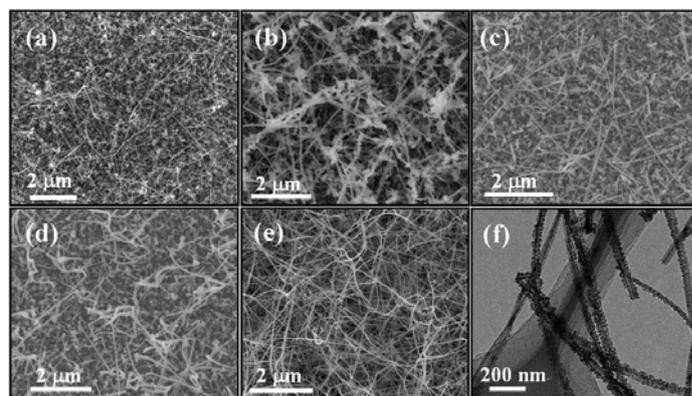
**Figure 1.** SEM images of GaAs NWs grown at source/substrate temperatures of: (a) 875/560 °C, (b) 875/600 °C, (c) 875/640 °C, (d) 850/600 °C and (e) 900/600 °C, and (f) is TEM image of (e). (H<sub>2</sub> flow rate of 200 sccm ~0.95 torr, growth time of 60 min)
