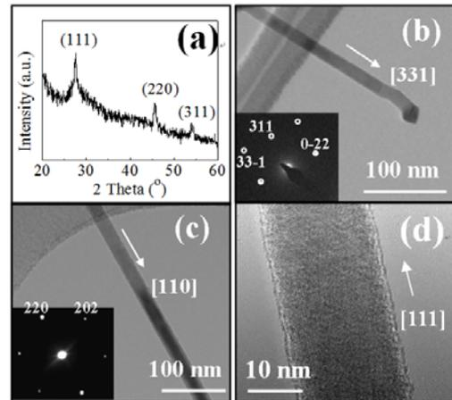
**Figure 3.** (a) is XRD pattern, (b) and (c) are TEM and SAED (zone axis of [-233] and [-111]) of GaAs NWs grown in [331] and [110] directions, and (d) is HRTEM image of NWs grown in <111> direction.
