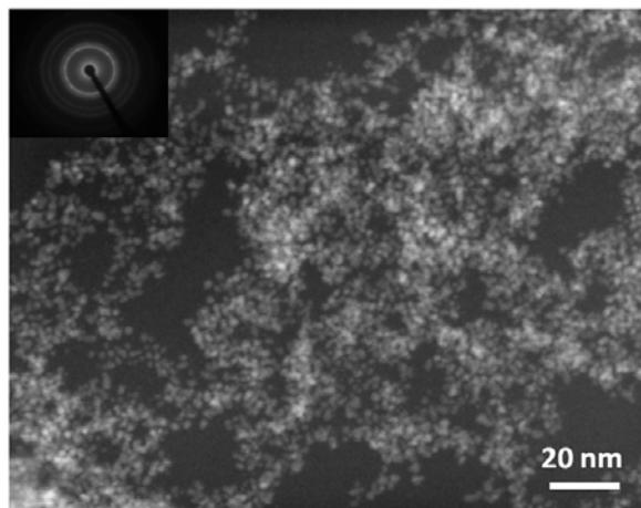
**Fig. 3.** A DF-TEM image of Pt nanoparticles prepared by *solution plasma sputtering*. Inset is the SAED pattern.
