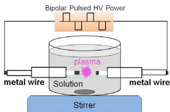
**Scheme 1.** Schematic diagram of the experimental setup by *solution plasma sputtering*.
