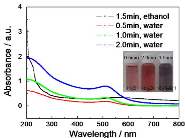
**Fig.2.** The UV-vis absorbance spectra of gold nanoparticles in water and ethanol, respectively. Inset is a photograph of gold nanoparticles solutions.
