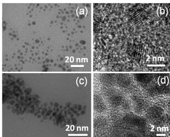
**Fig.1.** TEM (a, c) and typical HR-TEM images (b, d) of gold nanoparticles. (a, b) and (c, d) for samples prepared in water and ethanol medium, respectively.
