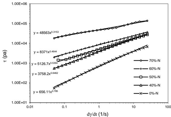
Fig. 2 Shear stresses versus shear rate according to Method 2
