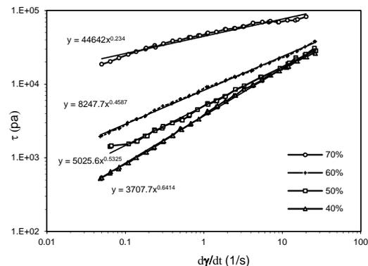
Fig. 1 Shear stresses versus shear rate according to Method 1
