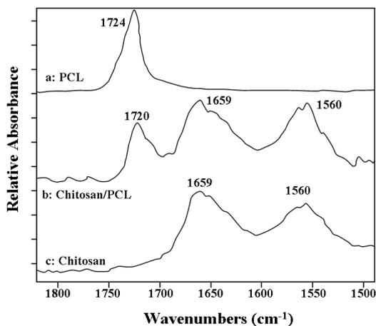
**Fig. 2** FTIR spectra of a: pure PCL; b: chitosan/PCL scaffold and c: pure chitosan
