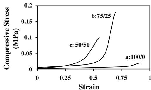
**Fig. 3** Stress-strain curves of chitosan/PCL composite scaffolds with different weight ratios a: 100/0, b: 75/25 and c: 50/50
