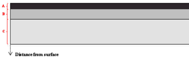
Fig.2 Schematic cross section of 2024 aluminum after SMAT treatment. (A, Nanocrystalline layer; B, Graded layer; C, Coarse grain.)
