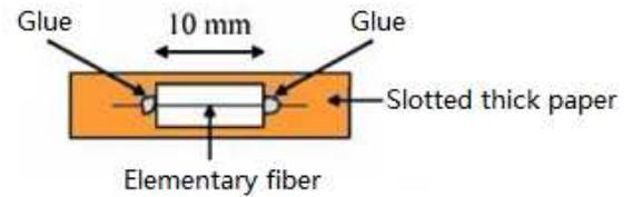
Fig.1 Illustration of individual testing sample.
