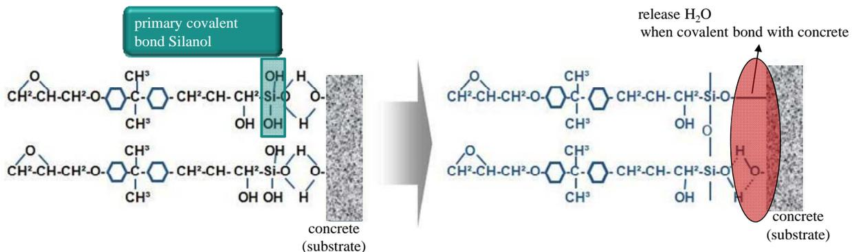
Fig. 1 Chemical bonding mechanism of non-shrinkage chemical grout (NCG)
