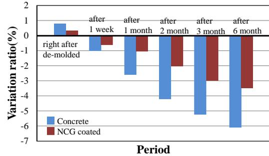
Fig. 5 Measured drying shrinkage of the specimen coated with NCG compared to conventional concrete
