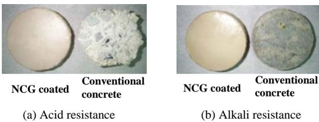
Fig. 2 Test results on acid and alkali resistances
