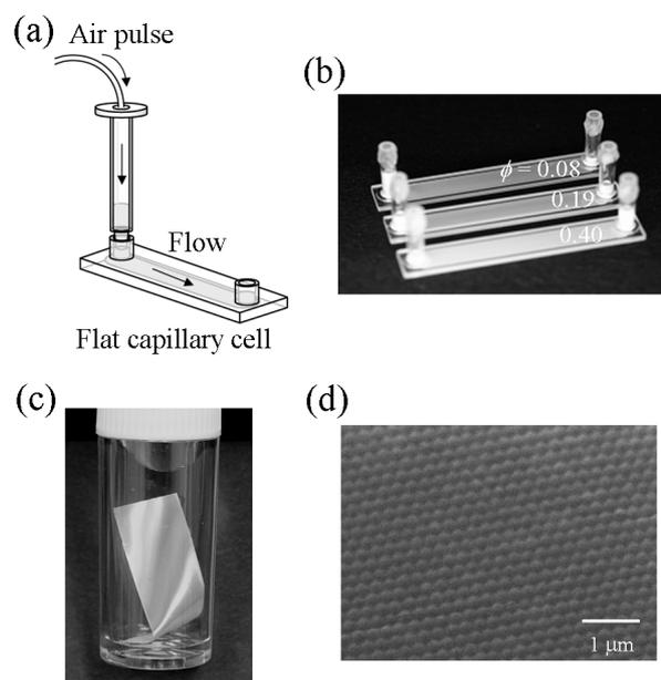
Figure 1 (a) Schematic diagram of the fabrication of a colloidal crystal film. (b) Photograph of flow-aligned colloidal crystal films with different particle concentrations. (c) Photograph of a gel-immobilized colloidal crystal film. (d) SEM image of dried colloidal crystal gel film.
