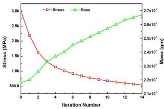
Fig. 3 Stress and mass optimization of an airbag inflator.
