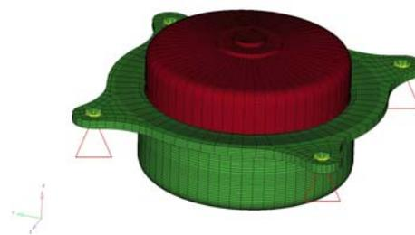
Fig. 1 Fine mesh and boundary conditions of an airbag inflator.
