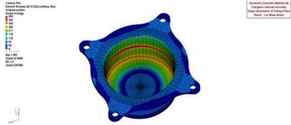
Fig. 5 von-Mises stress developed after 14<sup>th</sup> iteration
