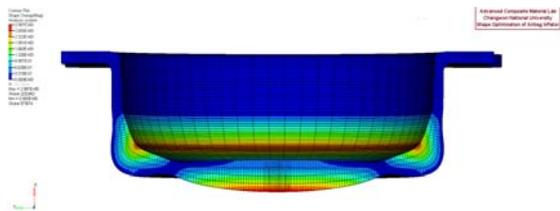
Fig. 4 Optimal shape of lower housing after 14<sup>th</sup> iteration
