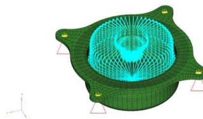
Fig. 2 Uniform distributed applied pressure during combustion.
