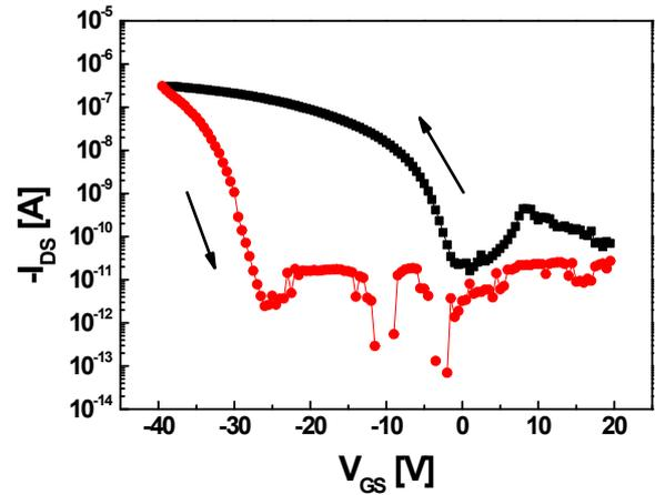
Fig 3. The I-V characteristic of the fabricated organic memory at different  $V_{GS}$  sweeping range.
