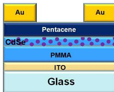
Fig 1. Schematic of the CdSe NPs/PMMA composition in the blend as the tunneling layer for non-volatile organic memory.
