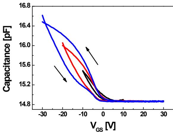
Fig 2. The C-V characteristic of the fabricated organic memory at different  $V_{GS}$  sweeping range.
