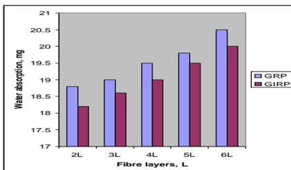
Figure 1, Relation between water absorption of GRP and GIRP against no. layers
