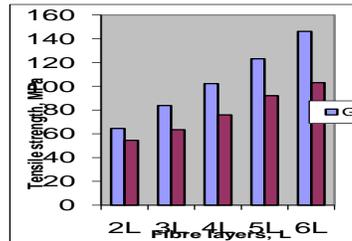
Figure 3: Variation in tensile strength of modified and unmodified cotton fibre-reinforced polyester with no. fibre layers
