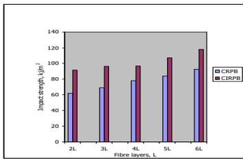
Figure 5. Variation in impact strength of modified and unmodified cotton fibre-reinforced polyester with no. fibre layers
