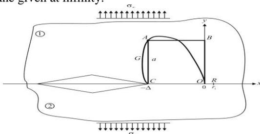
Fig. 1. Approximation of pre-fracture zone. Parameter  $r_i$  is specific linear size of a structure of the  $i$  th material. Let materials in the upper and lower half-planes differ only by limits of elasticity  $\sigma_{Y1} < \sigma_{Y2}$ . The sufficient criterion for mode I crack [4, 5]
