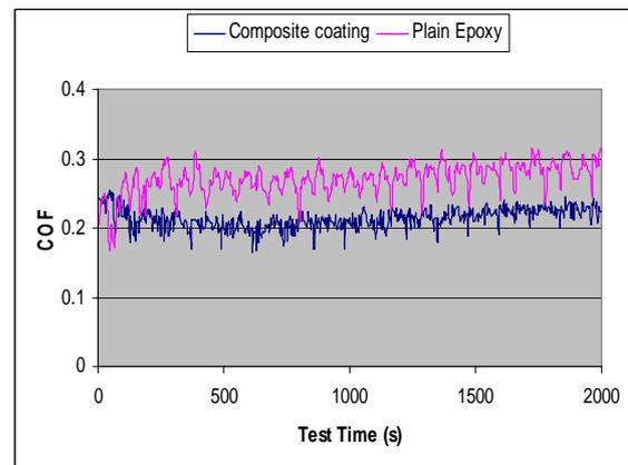
Figure 5 COF in tests under constant normal load with dia. 3mm ball on air-sprayed epoxy or epoxy-CNT composites, 16 cycles.
