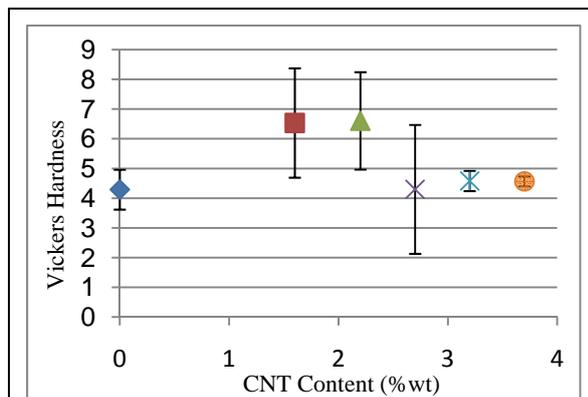
Figure 3 Effect of CNT content on the Vicker's hardness of composites
