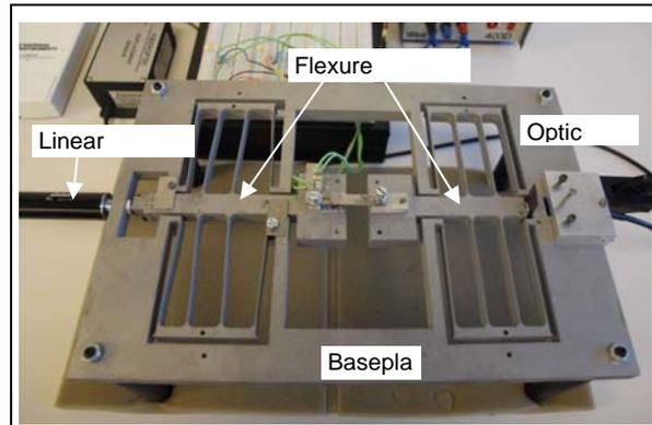
Figure 4 Friction test rig
