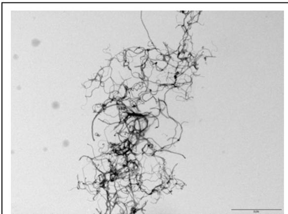
Figure 1: Multi-walled Carbon nanotubes
